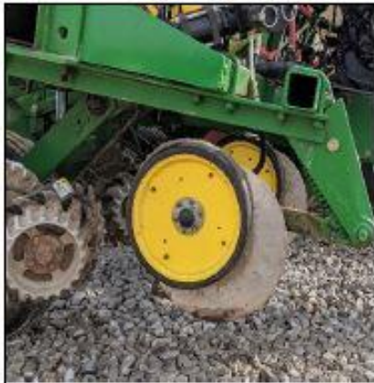
Figure 3. No-till corn planter with coulters for offset or 2x2 application provides an effective means to get N under surface residue.
